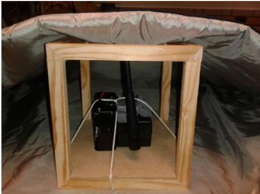
Fig. 3: Showing the comb completely covered by the Faraday bag
